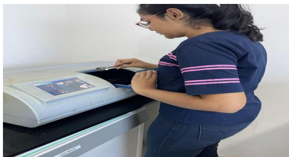
[Fig.5: Insertion of a Glass Polarimeter Tube (Containing Sample 1) into the Polarimeter]
